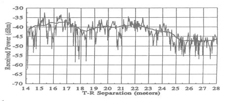
Fig.1 Typical plot of indoors Received RF Power versus range in meters [Rappaport, 2003]
